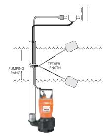
Pumping range determined by tether length according to the following guide.
